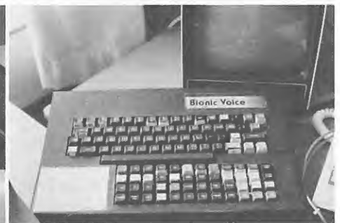
Rush's dorm room contains a typewriter with a switch mounted on top for turning on other appliances, a pushbutton telephone with an answering machine, and a voice synthesizer with a display screen.
