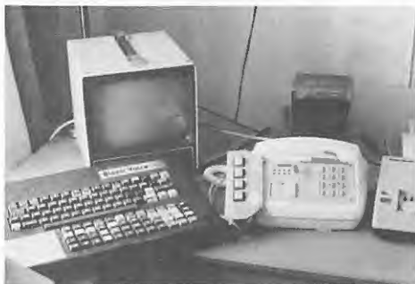
Rush's dorm room contains a typewriter with a switch mounted on top for turning on other appliances, a pushbutton telephone with an answering machine, and a voice synthesizer with a display screen.
