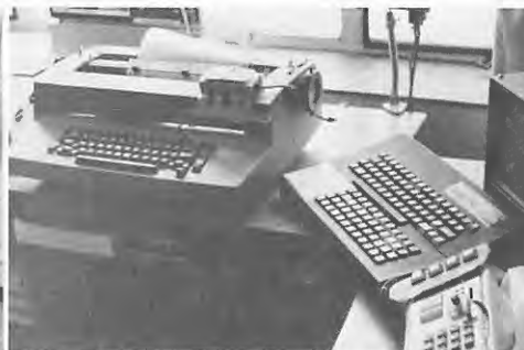
Rush's dorm room contains a typewriter with a switch mounted on top for turning on other appliances, a pushbutton telephone with an answering machine, and a voice synthesizer with a display screen.
