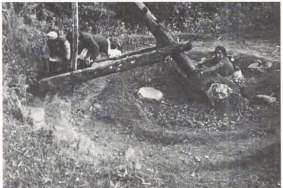
Villagers have constructed a simple wooden mustard-crushing instrument to use in preparing oil. In another village, superstition prevented construction of the crusher.
